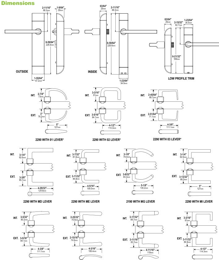
\* THE 2290-01, -02, AND -03 LEVER HANDLES ARE DESIGNED TO RETURN WITHIN 1/2" OF THE DOOR FACE. HANDLES IN THE DESIGNER SERIES DO NOT HAVE THIS SAME FEATURE. PLEASE VERIFY WITH LOCAL CODE REQUIREMENTS TO ENSURE COMPLIANCE.
